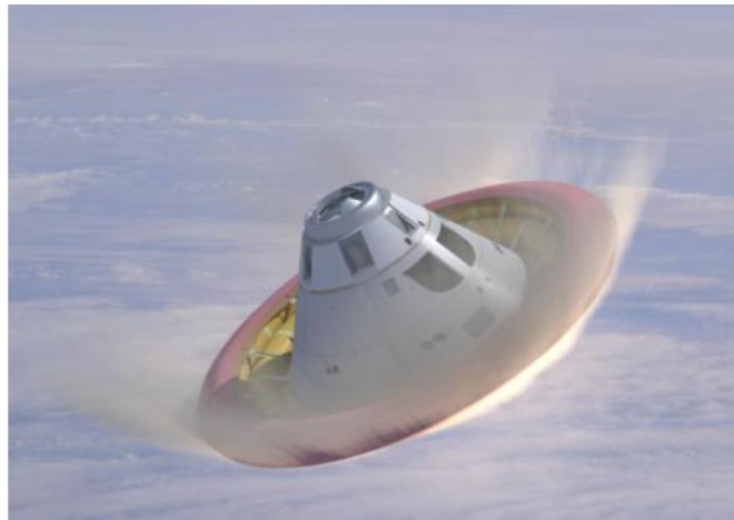
Figure 8: HIAD MAS Earth Entry Reference Vehicle [61]
