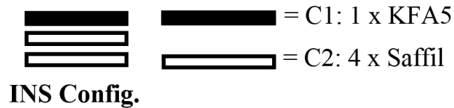
Figure 76: Sample FTPS Dual-Insulator Configuration
